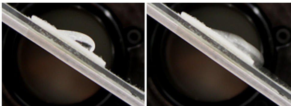
Fig. 15 Dodecane rolling off a superhydrophobic/superoleophobic surface
